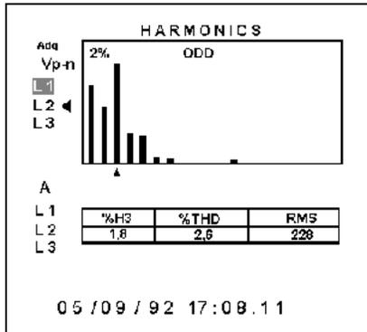
To view the percentage of distortion on the individual odd (or even) harmonic, use the left [◀], and right [▶] arrow buttons move the cursor [▲] along the bottom of the histogram.
