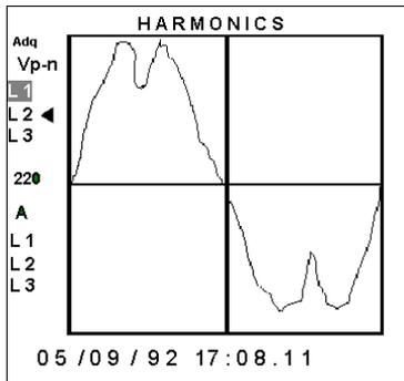
To capture new measurements on the waveform, use the up [▲] and down [▼] arrow buttons to move the cursor to the acquire icon [Adq] and press the enter [ENTER] button. The graphic representation of the new waveform will be displayed on the screen.
