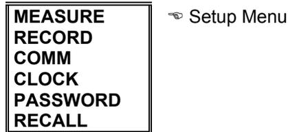
To enter a menu, use the up [**▲**] and down [**▼**] arrow buttons to move through the available parameters and press the enter [**ENTER**] button.
