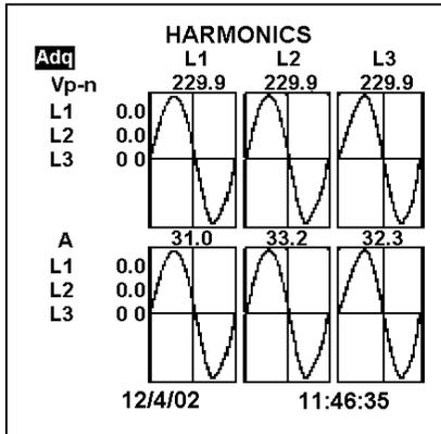
There are two additional screens that can be accessed from the scope view screen, the waveform zoom and the harmonic bar graph screens. These give additional information on the shape of the distortion and the harmonic content causing the distortion.
