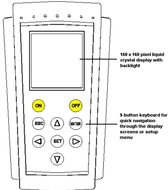
For best viewing in direct sunlight, or in dark areas, the user can adjust the display contrast. Use the left [ ◀ ] and right [ ▶ ] arrow buttons to increase or decrease the display contrast. The contrast will change while you are making the adjustment. This can also be changed from the programming menu. See section 5.3.3 of this instruction manual for more information.
